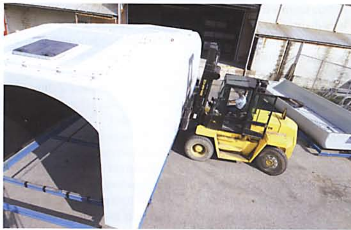
McClarin Plastics Inc. employee David Frock moves a wind turbine nacelle into the shipping yard at the company's renewable-energy division in York County. The fiberglass components will be transported to wind-farm developer Gamesa's Bucks County facility for assembly.
