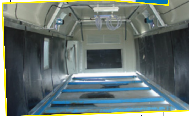
Interior shot of the spinner nose hub that McClarin produces for Gamesa. The piece is made of fiberglass using the vacuum infusion method.
